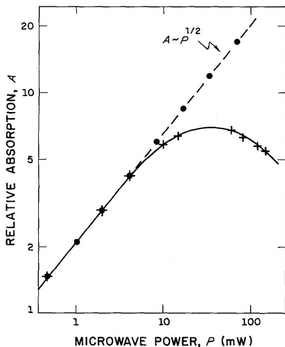
Figure 3 Microwave absorption as a function of microwave power for two high-temperature superconductors: (●) Bi-Sr-Ca-Cu-O, present work; (+) Y-Ba-Cu-O [14].
