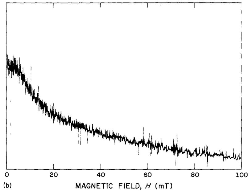
Figure 1 Microwave absorption derivative spectrum of the Bi-Sr-Ca-Cu-O system at 77 K. (a) Spectrum taken with the field increasing from 5 to 100 mT; (b) spectrum taken with the field decreasing from 100 to 5 mT. The experimental parameters are microwave power 15 mW; microwave frequency 9.1 GHz; modulation amplitude, 10  $\mu$ T.
