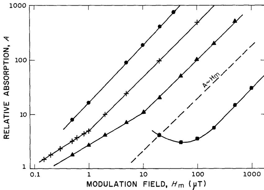
Figure 2 Microwave absorption as a function of modulation field amplitude for several high-temperature superconductors: (●) Bi-Sr-Ca-Cu-O, present work; (+) Ba-La-Cu-O, (▲) La-Sr-Cu-O and (■) Y-Ba-Cu-O [13].
